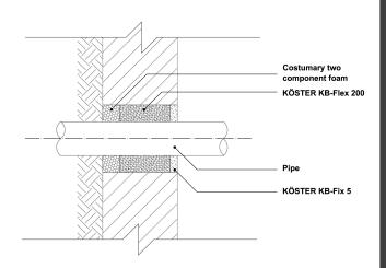
When sealing cable penetrations, jiggle the cables to reveal voids and re-press KÖSTER KB-Flex 200 into any eventual voids created. Ensure that the cable is tension free after finishing the sealing. Finally the sealing compound is recessed 1 - 5 cm (depending on cable thickness and weight) from the wall surface and smoothed with a metal spatula. As an additional safeguard and to hold the pipe / cable centered, the exposed material is covered with KÖSTER KB-Fix 5.
